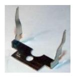
6.13 Fold up the correct replacement guard irons, [T3] for Deeley tender, [T4] for Fowler tender, by firstly bending the two guard irons at right angles and then bend the straight sections to a lazy 'S' shape (see prototype photo of a Fowler tender with steam heating pipe). Finally file off the two small tabs between the guard irons. (see photo). Note – these tabs should not be removed if you are intending to use the replacement footplate (see section 10)
