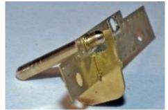
7.3.9 Replace the Bachmann buffers or fit replacement buffers, undoubtedly you will have damaged the Bachmann red paint so it is probably best to remove this from all the buffer body before re-fitting.
