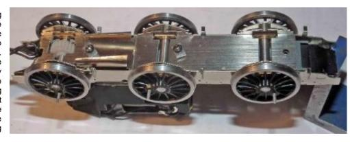
5.16 Push through the four rivets in each guard iron [**L4** and **L5**] and form to a slight 'S' shape. Glue or solder to the chassis frames immediately in front of the leading axle brake 'pockets' (there is a mark on the frames) with the curved face leading.
