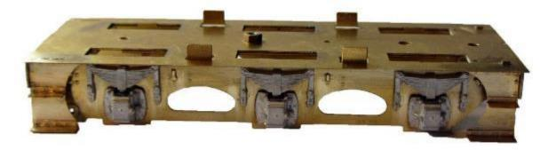
12.2.39 If using with the EasiChas tender frames, solder a 10 BA nut in the recess on the top of the tender base [FF5].
