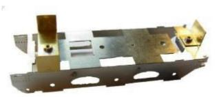
using 10 BA screws, the Ushaped bracket [FF10] at the front, the L-shaped bracket [FF11] to the rear (see photo). Using epoxy resin on the inside of the tender sides and back, attach the brackets to the tender body by positioning
