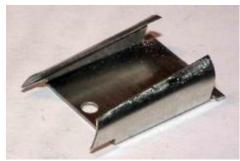
drivers can be obtained by having the thin side of the bearings on the outside or rubbing off the circular beading round the axle hole. For EM gauge, it will be necessary to file off the raised rim on the inside face of the bearings to ensure the bearings move up and down freely.
