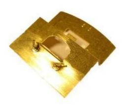
11.3.23 Make a right angled bend in two pieces of 0.33 mm wire and thread through the two holes in the lower half of the tender front from the back, ensuring they are perpendicular. Solder the valve bodies [FD19] over the wire to the front of the tender front, ensuring that they are correctly orientated (see photo).
