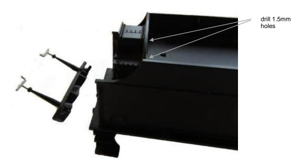
11.3.4 Drill two holes about 1.5 mm immediately behind the front coal partition and close to the outside of the coal space (see photo above)
