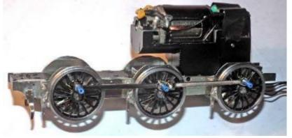
damage the gears if allowed to repeatedly occur. Even though theoretically impossible the front springs can disappear from a completed loco. A drop of 5 minute epoxy at their extreme top where they bear onto the chassis will secure them – trust us on this one!
