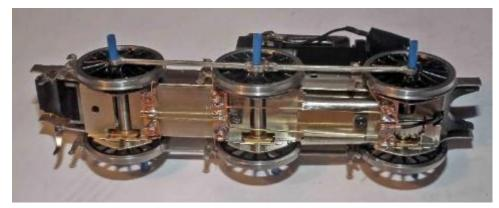
5.22 Glue the pick-ups to the chassis keeper plate in the position shown in the photo so they gently press onto the wheel flanges. Test the polarity and direction of travel with another loco and connect together with brass wire and to the motor with wire. Test run with and without the body fitted. When happy, remove the temporary crank pins, shorten the bushes and fit the crankpin bushes (note, if you are going to fit new coupling rods as per section 7.1 do **NOT** shorten the bushes).
