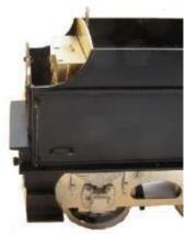
12.1.12 Refit the Bachmann brake hangers, having modified them first if required (see section 11.1), securing in place through the holes in the tender frame with cyanoacrylate glue or epoxy resin.
