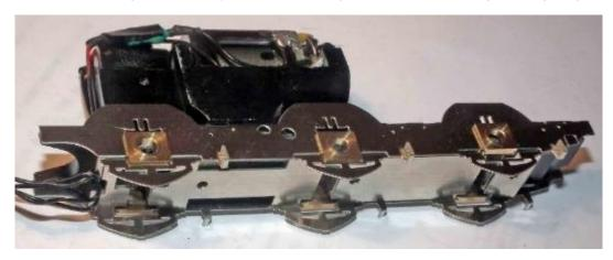
5.8 Using about a 3mm diameter rod (or an axle or even the shank of a jewellers screwdriver) as a former, curve up the half-etched sides of the ash pan [L3] with the half-etch to the inside. Fold up the ashpan into an inverted U with the side curving in towards the middle. See photo. The ashpan is screwed under the keeper plate with the two 'ears' keeping it central. See later photos.
