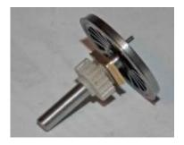
on each side of the leading and trailing wheels, and finally press the wheels on the axles.
