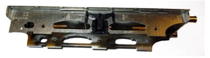
10.20 Cut the axlebox and spring hanger assemblies from the Bachmann frames using a piercing saw. Trim around the axlebox and spring. Remove the raised section on the back of the moulding and then attach to the replacement frames using cyanoacrylate glue or epoxy resin (see photo above).
