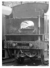
11.3.25 Push through the rivets in the top half of the new front for the fire iron bracket and, if being fitted, the rivets for the coal rails.
