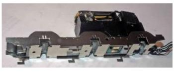
5.4 Ensure the mainframes fit over the original Bachmann chassis. The frames should sit parallel to the Bachmann frames and not be 'splayed' out at the top. If necessary file the top strips back to ensure this. See Photo. Remove the mainframes.
