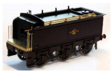
9.3.19 If fitting to the Bachmann tender frames, extend the slots in the Bachmann tender frames that receive the hooks at the front of the tender top towards the rear of the tender so that the tender top can be inserted without tilting so far. This enables the top to be taken on and off without damaging the handrails.
