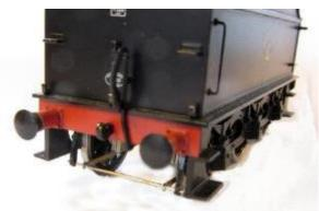
11.2.7 Remove the brake pull rod assembly and put to one side until all the work on the tender is complete. When it is attach the pull rod assembly to the plastic brake gear using cyanoacrylate glue or epoxy resin.
