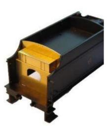
11.3.13 The toolbox and toolbox top have been deliberately left slightly over-long, so now file them back flush with the toolbox ends. Similarly, the toolbox ends are slightly over long so the back edge now needs filing back to match the toolbox top and to allow the toolbox to sit back against the tender front.
