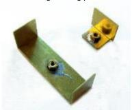
12.1.6 Solder 10 BA nuts to the half-etched recesses in the top of the tender sideframes [FF1] and the two mounting brackets [FF10
