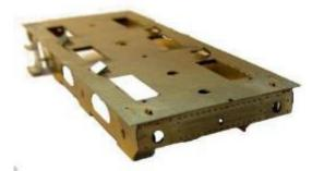
12.2.12 There are two different types of drag beam, with a rounded end [FF6 and FF7] and the later type with an angled end [FF8 and FF9]. Push
