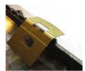
11.3.6 Take the new tender front [FD12] and identify the large half-etched section where the large radius curve will be formed. This section needs to be bent around a 2.8 mm drill
