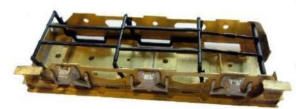
12.2.45 If using the replacement brake pull rods, assemble them in accordance with section 11.2 then cut the brake shaft from the pull rods as shown in the photograph.
