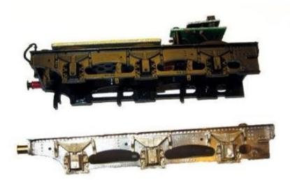
10.18 Attach the buffers to the buffer beams on the replacement frames using cyanoacrylate glue or epoxy resin.
