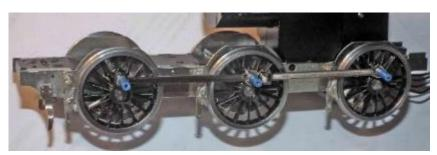
7.2.6 Attach the brake hangers to the wire, making sure that the brake blocks do not touch the wheels, which would cause a short circuit. Attach the brake hanger bracket outer etches, [L37] for left hand side, [L38] for the right hand side, over the wire on the outside of the brake hangers and solder in place. If you get flux on the treads of the wheels they will rust – we protect them with a thin bit of masking tape during this process.
