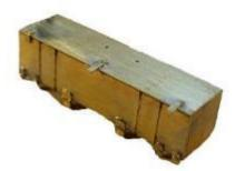
11.3.19 Bend the overhanging part of each hasp and staple down over the front of the tool box, ensuring it lies flat with the front (see photo).
