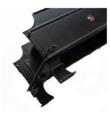
11.3.9 Check the fit of the front in the Bachmann body. You will probably find that where the old front was cut away the sides are thicker than the part in front. This thick part need to be cut and filed back until the front sits back so that the distance from the front edge of the tender sides to the new front is 5.66 mm and the new front is vertical.
