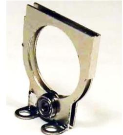
Adjust the components of the drive shaft so that it just extends beyond the rear ball bearing and the gear is central to the gap in the front motor mount. Loctite the sleeve of the gear to the drive shaft. Making sure that the ball bearings are fully pushed home in their sockets, apply a small amount of Superglue to the ball bearings so that it runs into the gap to hold them permanently in place. The drive shaft should spin freely.
