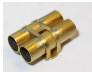
8.2.4 Bend up the retaining straps [D9], cut the legs to the correct length and solder in position. See photo.
