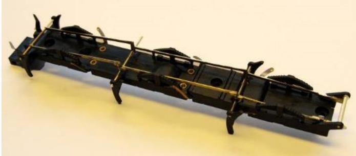
4.1.15 Refit the keeper plate to the loco chassis using the original screws.
