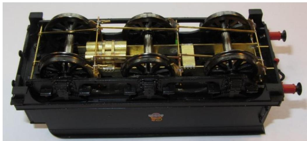
8.3.11 Refit the Bachmann wheels and check that the brake hangers are in the correct position across the face of the wheels. If not, adjust either the 0.5 mm cross shaft or the small piece of tube on the cross wire, or both.
