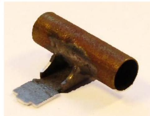
8.2.5 Solder the support bracket into the cutouts in the frame between the leading and centre wheels with the 5 mm overhang towards the front of the tender.
