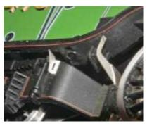
6.4 Fold the smaller bracket [D15 and D16] to 90 degrees along the slots with the bolt detail on the inside of the bend and fit to the Cartazzi truck frame immediately in front of the moulded spring hanger in-line with the rivets and with the riveted flange towards the front of the loco (see photo above). Fix using cyanoacrylate or preferably epoxy resin (the plastic is difficult to fix to and fixing is helped by scoring the plastic).
