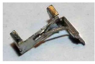
5.5 Bend the step supports as shown in photo left, making the bends at the end of the half etched section and at the small hole in the half etched section. Solder to the base of the footsteps. See photo right.
