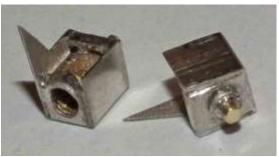
4.8 Cut two short lengths of 1.0 mm diameter wire. Insert the wire through the buffer washer [D8] and the smaller hole in the end of the buffer spring housings ensuring that the wire does not protrude into the tube. Trim the wire to length. Solder together (see photo of the finished assemblies).
