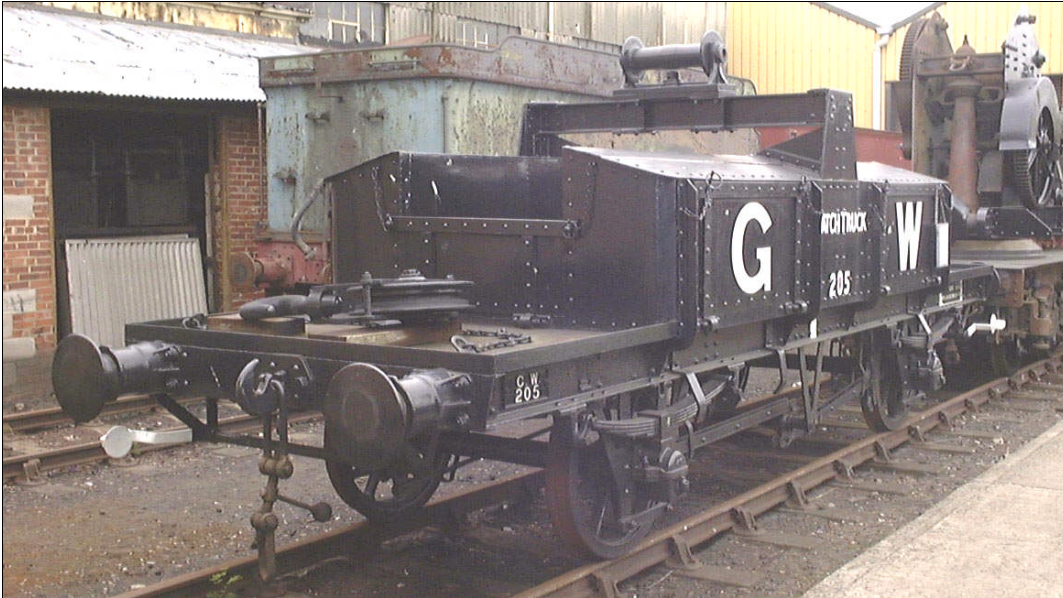
Fig.1 No. 205 at Didcot, illustrating the general appearance of a match truck. Note the welded floor and backs of the toolboxes, square corners to the corner angles, floor rollers removed, riveted toolbox roof and other fittings added, tapered ends to headstocks, and several other variations from the L.4 vehicle as built.
