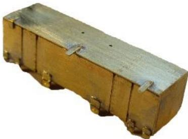
11.1.20 Using 0.33 mm wire bend up the handrail on the top of the toolbox and solder in place
