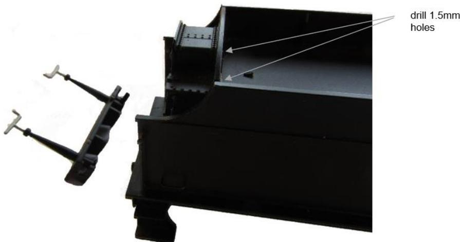
11.1.4 Drill two holes about 1.5 mm immediately behind the front coal partition and close to the outside of the coal space (see photo above)
