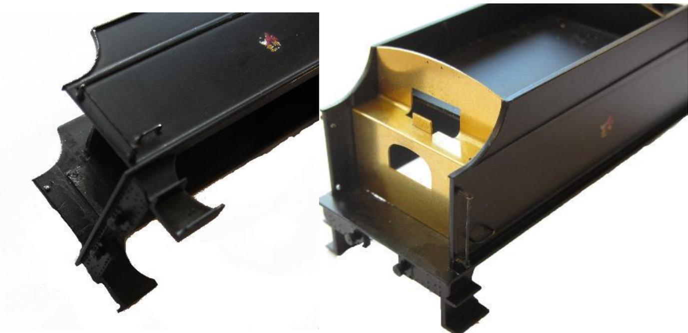
11.1.10 Push through the rivets in the toolbox [2] and the tool box top [3]. Fold up the tool box [FD13] into a U shape making sure the bends are 90 degrees.
