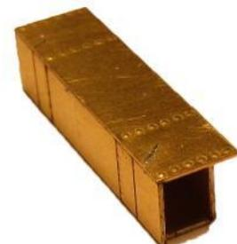
11.1.13 The toolbox and toolbox top have been deliberately left slightly over-long, so now file them back flush with the toolbox ends. Similarly, the toolbox ends are slightly over long so the back edge now needs filing back to match the toolbox top and to allow the toolbox to sit back against the tender front.
