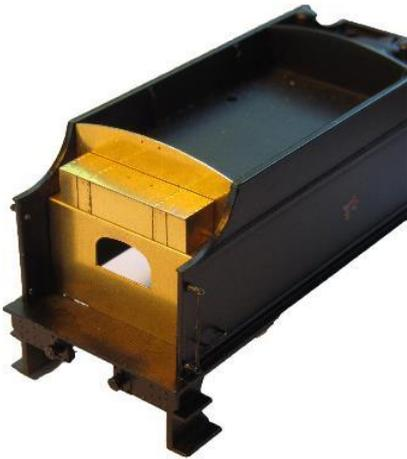
11.1.14 Now the fun begins. It is time to solder on the hinges and the hasps and staples. We have managed to make this easier for you in the production etch than in the first test etch by attaching the components on strips with guides.
