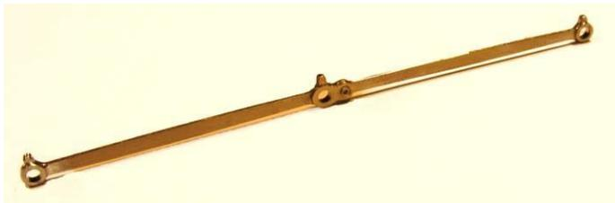
9. Open up the crankpin holes in order that the rod will either rotate on the crankpin screw (if using Bachmann wheels) or on the crankpin bushes (if using Alan Gibson or Ultrascale wheels). This can be done with a reamer, broach or a fine Swiss file.
