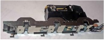
5.4 Ensure the mainframes fit over the original Bachmann chassis. The frames should sit parallel to the Bachmann frames and not be 'splayed' out at the top. If necessary file the top strips back to ensure this. See Photo. Remove the mainframes.
