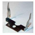
6.11 Fold up the correct replacement guard irons, [T3] for Deeley tender, [T4] for Fowler tender, by firstly bending the two guard irons at right angles and then bend the straight sections to a lazy 'S' shape (see prototype photo of a Fowler tender with steam heating pipe). Finally file off the two small tabs between the guard irons. (see photo). Note – these tabs should not be removed if you are intending to use the replacement footplate (see section 10)
