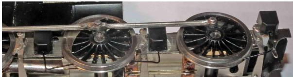
5.46 Attach the centre and trailing sandboxes to the mainframes using cyanoacrylate glue or epoxy resin. There are two small indentations on the mainframes where the top corners of the sandbox should be located; they do not sit flush with the tops of the frames.
