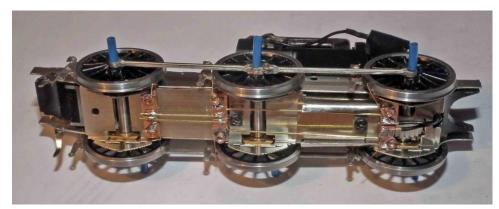
5.22 Glue the pick-ups to the chassis keeper plate in the position shown in the photo so they gently press onto the wheel flanges. Test the polarity and direction of travel with another loco and connect together with brass wire and to the motor with wire. Test run with and without the body fitted. When happy, remove the temporary crank pins, shorten the bushes and fit the crankpin bushes (note, if you are going to fit new coupling rods as per section 7.1 do **NOT** shorten the bushes).
