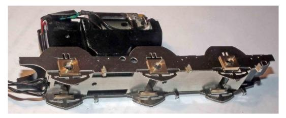
5.8 Using about a 3mm diameter rod (or an axle or even the shank of a jewellers screwdriver) as a former, curve up the half-etched sides of the ash pan [L3] with the half-etch to the inside. Fold up the ashpan into an inverted U with the side curving in towards the middle. See photo. The ashpan is screwed under the keeper plate with the two 'ears' keeping it central. See later photos.
