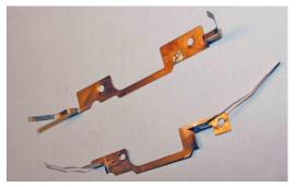
13.3 Using two 12 BA screws and nuts fasten the pickup strip back into position on the Bachman tender frames. Adjust the pickups so that they bear on the backs of the leading and trailing wheels. Check that there are no shorts between the pickups and the EasiChas tender frames.
