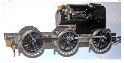
Even though theoretically impossible the front springs can disappear from a completed loco. A drop of 5 minute epoxy at their extreme top where they bear onto the chassis will secure them – trust us on this one!
