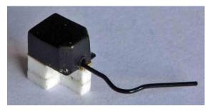
5.39 The leading sandboxes were quite wide extending beyond the face of the wheels and the coupling rods. Join a piece of 4 mm x 2 mm plastic strip to a piece of 4 mm x 1 mm and a piece of 4 mm x 0.25 mm, all 7 mm long, using solvent, to form a spacer block.
