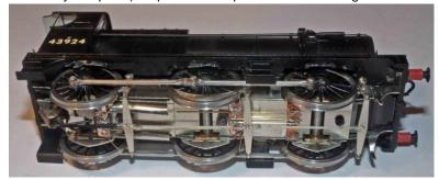
as a positioning guide (see <a href="www.rail-online.co.uk">www.rail-online.co.uk</a> for a selection of over 200 MR and LMS 4F photos) The large balance weight sits on the middle driven axles' wheels but offset by one spoke, the two smaller weights are for the outer wheels exactly opposite to the crankpin boss.
